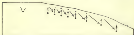
FIG. 159.—Diagram to illustrate the movements of soil particles due to freezing and thawing on level and on steep slopes.
